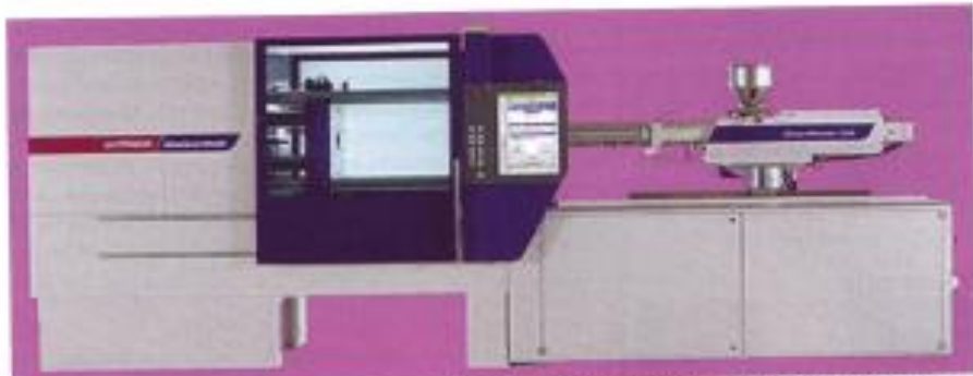
A servo-hydraulic injection molding machine. The Fig. 1A flow chart below illustrates the POSy-System methodology.
